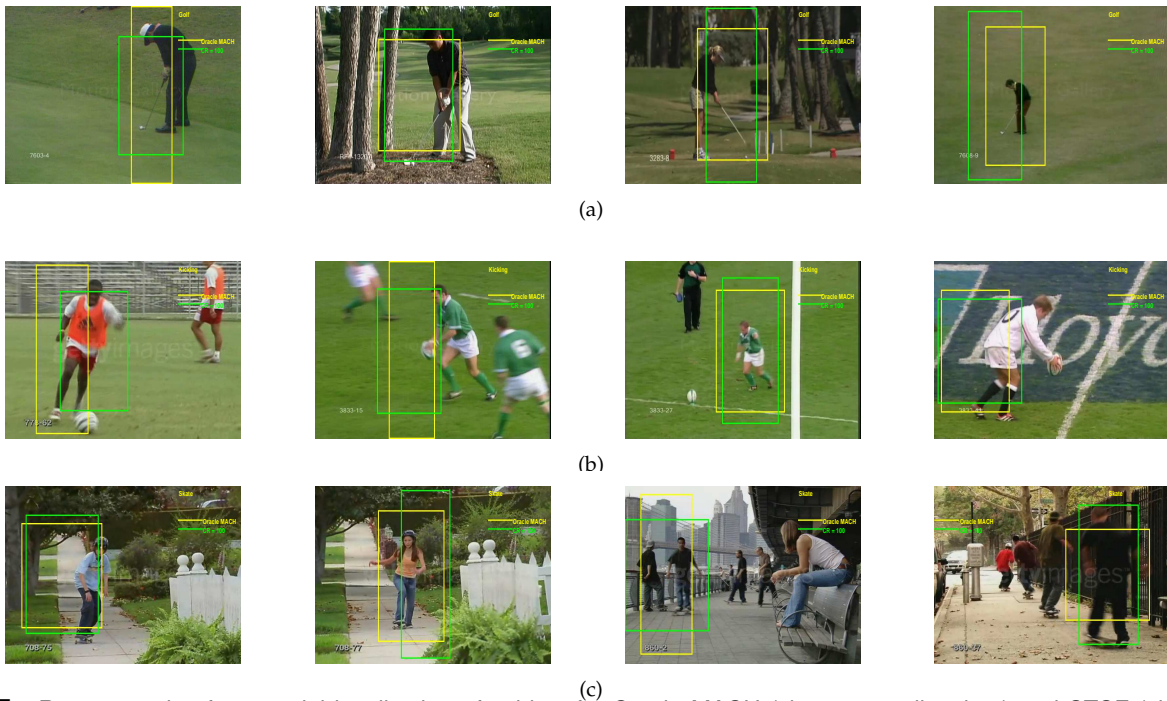
Fig. 7. Reconstruction-free spatial localization of subject for Oracle MACH (shown as yellow box) and STSF (shown as green box) at compression ratio = 100 for some correctly classified instances of various actions in the UCF sports dataset. a) Golf b) Kicking c) Skate-Boarding. Action localization is estimated reasonably well directly from CS measurements even though the measurements themselves do not bear any explicit information regarding pixel locations.
